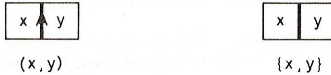
Figure 5.1. Oriented (x, y) , and unoriented \{x, y\} edge-elements.
