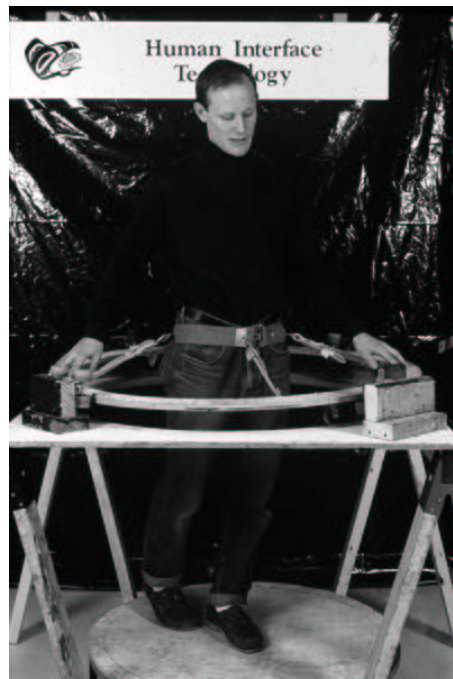
FIG. 2.11 – Le Virtual Motion Controller , un tapis muni de capteurs, copyright Human Interface Technology Lab, Washington
